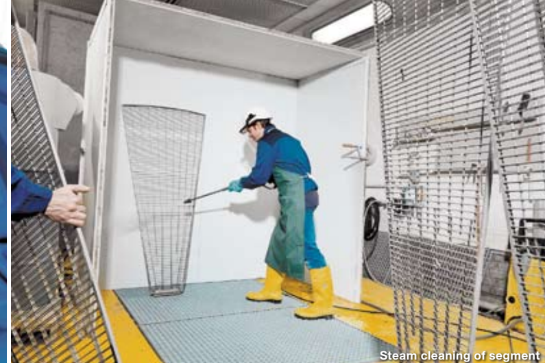
Steam cleaning of segment
