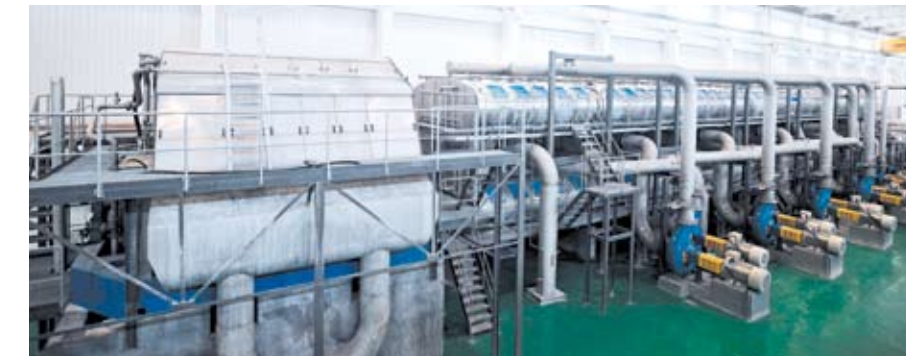
ANDRITZ delivered totally three SelectaFlot flotation stages to obtain maximum final pulp quality. ▶
