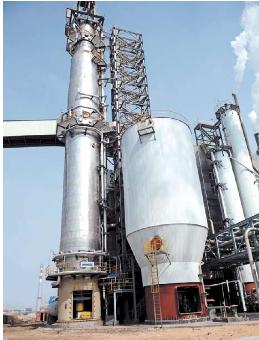
▲ Lower section of ANDRITZ Diamondback chip bin
