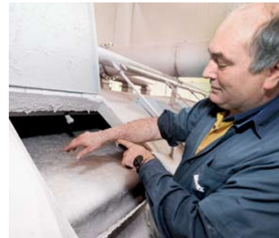
ANDRITZ delivered totally three SelectaFlot flotation stages to obtain maximum final pulp quality. ▶
