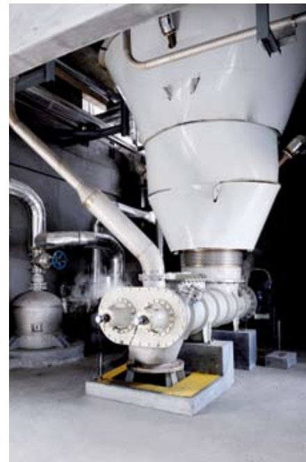
▲ Lower section of ANDRITZ Diamondback chip bin
