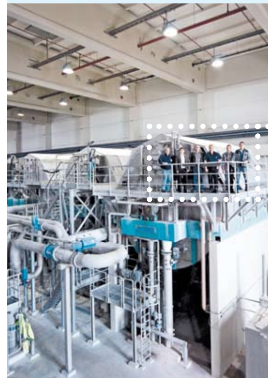
◀ Three ANDRITZ disc filters in the DIP plant at Augsburg. The two remaining units are installed as saveall fiber recovery filters for PM3.
