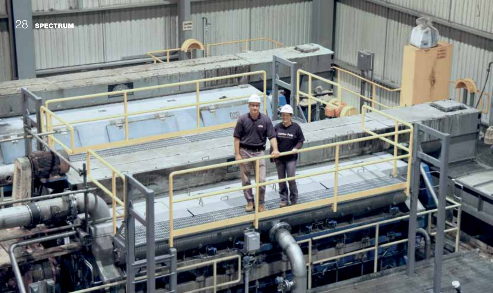
▲ Greg Hallas, ANDRITZ Product Manager for Twin Roll Press Services (left), with Kelly Parfitt, Canfor Project Engineer, standing on post-oxygen press #1 that received the Mult-E-Nip upgrade.
