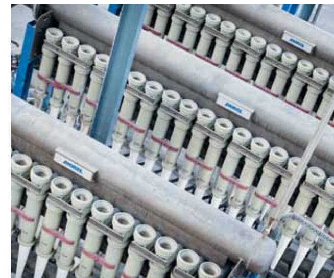
▲ After pulping, the next task is the removal of heavy particles in a two-stage cleaning system, preserving the life of downstream equipment.
