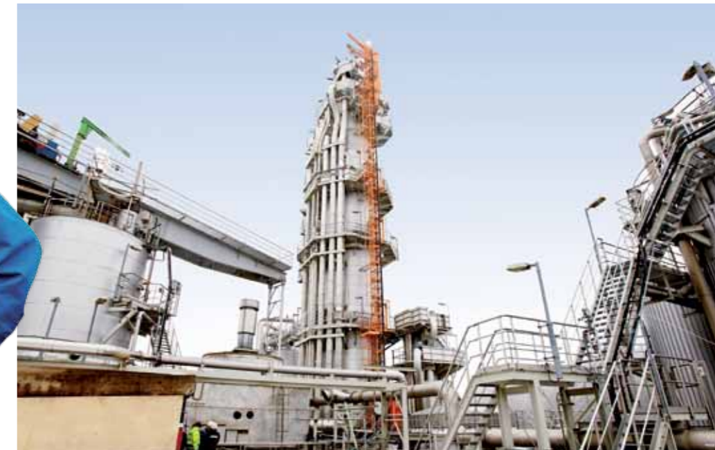
▲ ZPR now gets about 100 t/d more production out of its digester as a result of several small improvement projects. The most recent upgrade to the fiberline was the replacement of the lower extraction screens with new ANDRITZ SureFlow diagonal screens.
