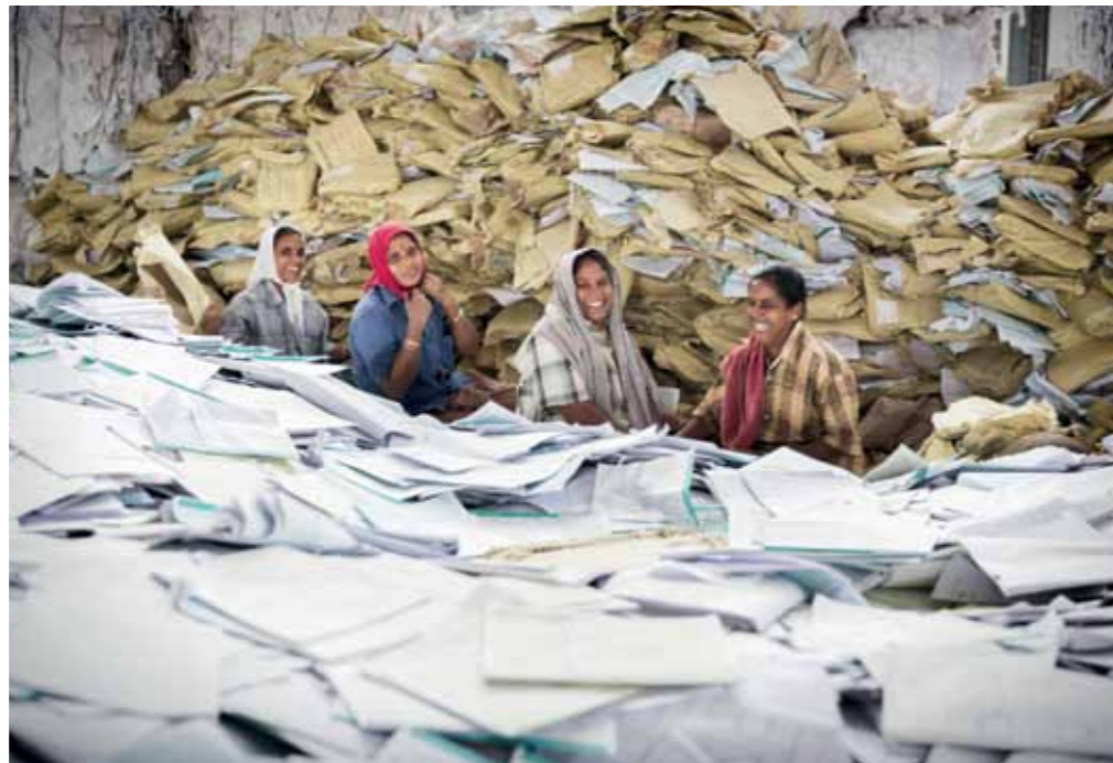
▲ The raw material mix consists of 80% sorted office paper and 20% old magazines. The ANDRITZ deinking and bleaching technology achieves a final brightness up to 87% ISO.
