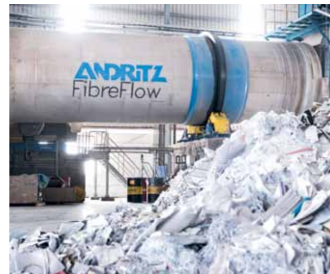
▲ The FibreFlow drum pulper is considered a core technology in the DIP line by TNPL management. It disintegrates the secondary fibers without harming them, while large contaminants are removed intact.
