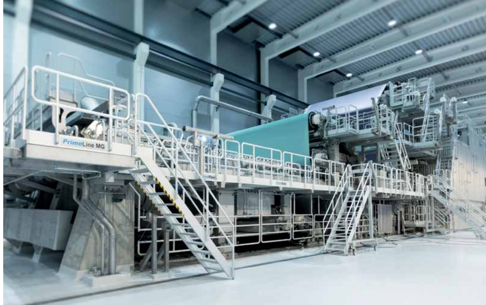
▲ The PrimeLine MG paper machine has a working width of 5.4 m and features a number of technical highlights.
