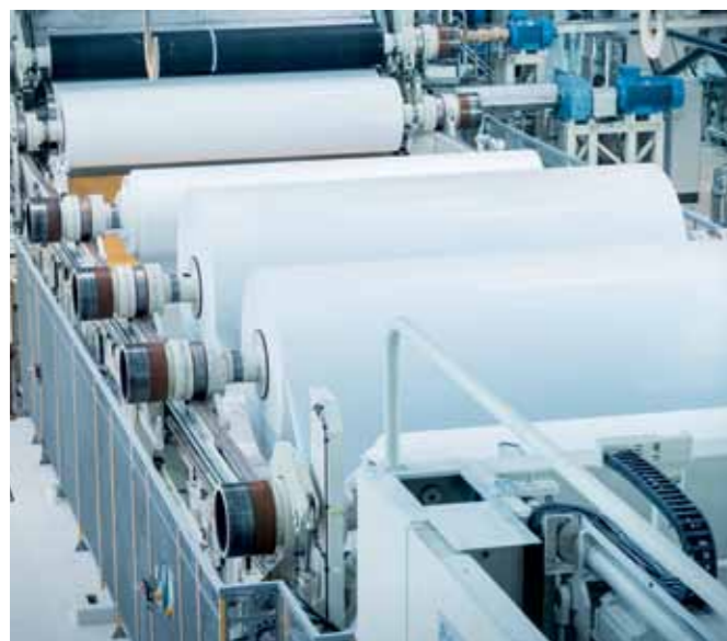
▲ The jumbo reel is rewound and converted to rolls on a two-drum PrimeWinder Arcus Evo.
