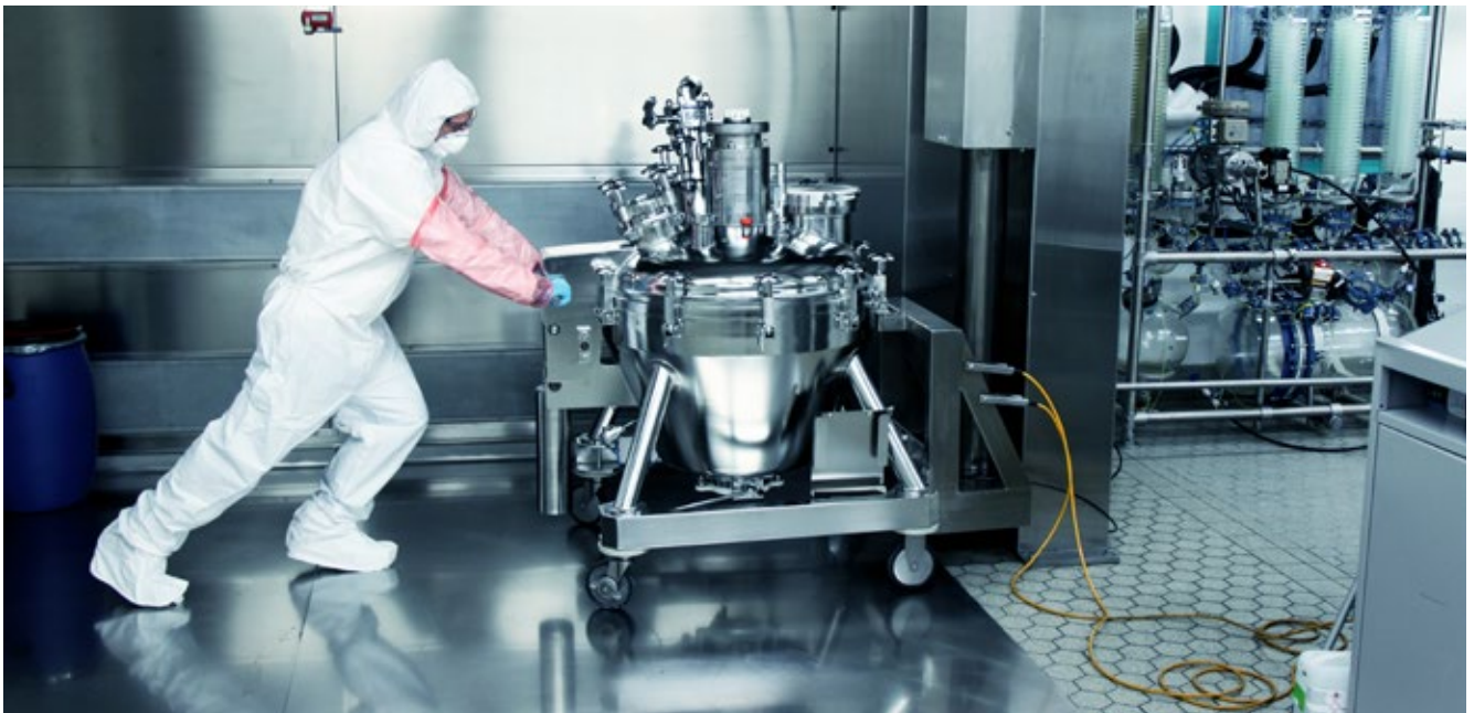
Filling, transport and product discharge with one single mobile dryer.
